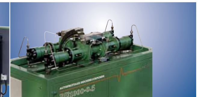
ULTRA HIGH PRESSURE PUMPS and components for autofrettage and pressure testing units with operating pressures of up to 1,000 MPa with a flow rate of up to 0.5 l/min.
