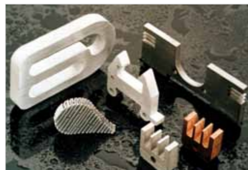
Technical parts, cut with an abrasive waterjet.
