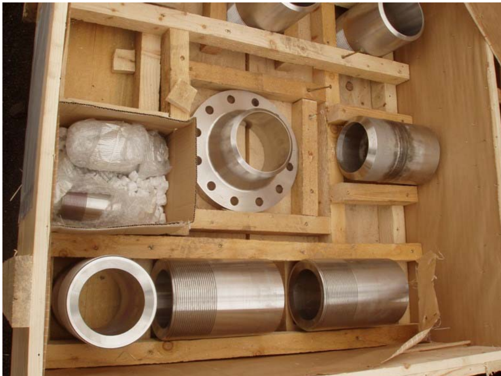
and various High Pressure pipe fittings in Safurex ® material were delivered at site.
